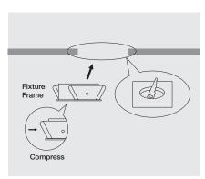
Cutout and compress spring plates to insert fixture frame to ceiling.
