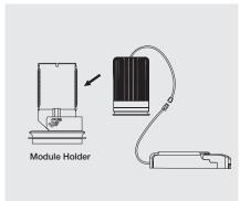
Attach module to module holder with spring clip and connect module to driver.
